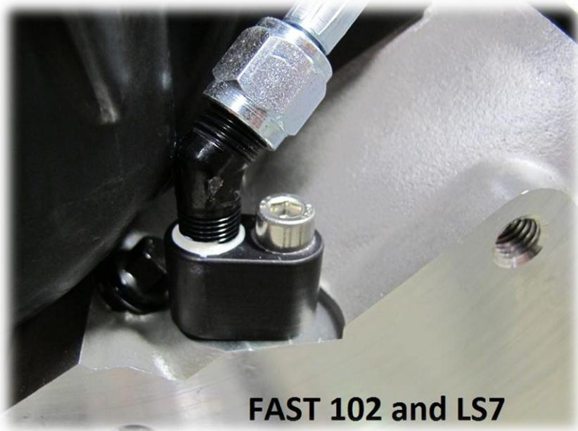
3. Secure a water line adapter to each steam vent on the cylinder heads using one of the supplied stainless bolts (anti-seize is recommended on these bolts). After the adapters have been secured to the heads, go ahead and tighten the -4an fittings.
