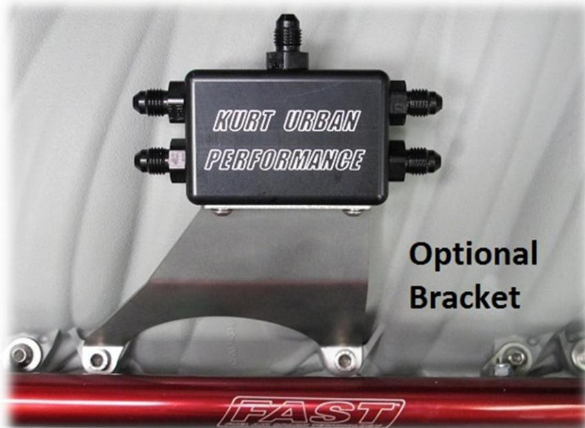
NOTE: When mounting the bracket, the washers for the intake bolts do not need to be used as they may interfere with the bracket.
