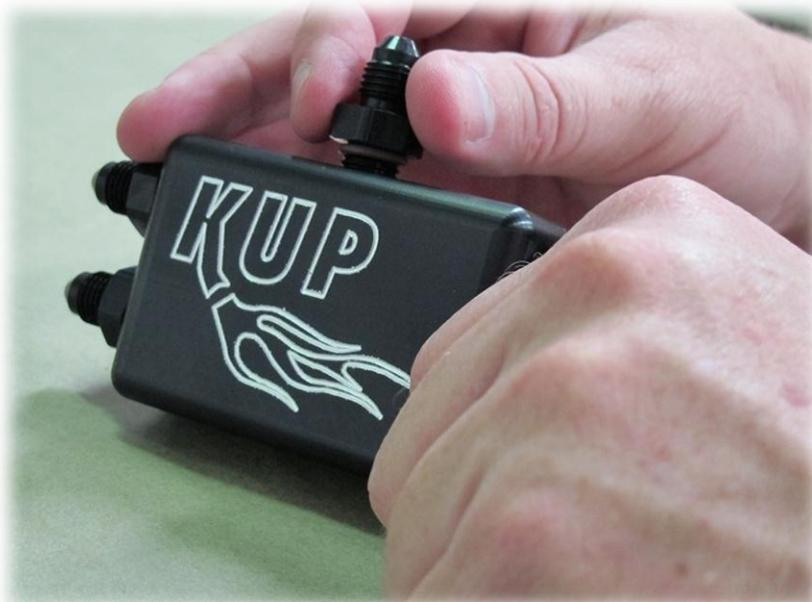
6. Attach the four provided lines to the collection block as shown. The remaining fitting on top should be plumbed back into your cooling system at the highest point possible. This may be back into the radiator below the cap, or possibly into an expansion tank. Another option is to drill the factory style water pump and return the line there with the appropriate fitting. We do not supply the lines and fittings for this as every application is different.
